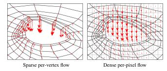
**Figure 9:** We efficiently convert sparse per-vertex image-space flows (left) to a dense per-pixel flow field (right) using GPU rasterization. We use this dense flow-field to warp the eyelids.
