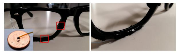
Fig. 2. Fully integrated version of *InvisibleEye* consisting of multiple, millimetre-size Awiba NanEye RGB cameras (marked in red) that are invisibly integrated into an off-the-shelf glasses frame. For our evaluations we developed two other prototypes to be able to characterise performance across key design parameters, including image resolution and number of cameras, as well as camera angle and positioning, and to compare with a state-of-the-art (high-resolution) mobile eye tracker.
