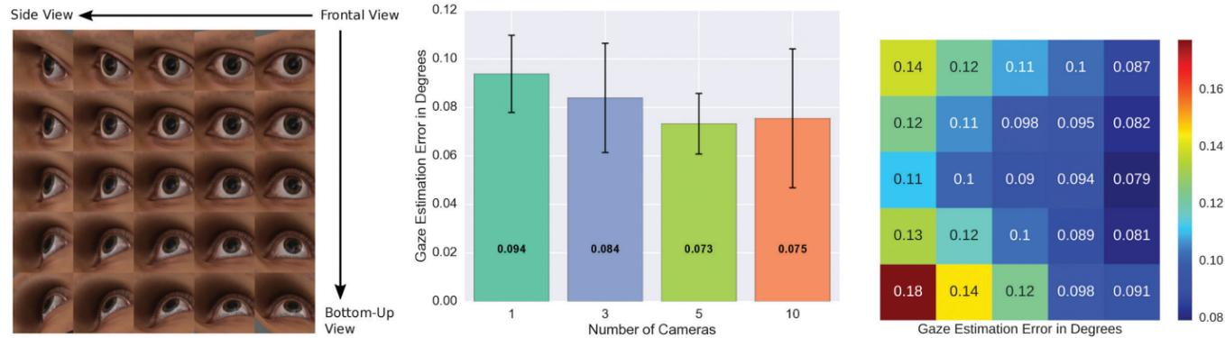
**FIGURE 2.** The use of synthetic images (left) allows us to evaluate the performance for a varying number of cameras at 5x5-pixel resolution (middle) as well as a wide range of camera angles (right) measuring the average gaze estimation in degrees.
