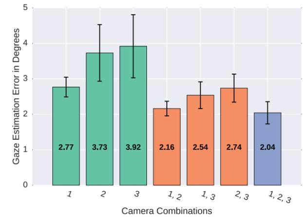
**FIGURE 4.** (Top) Second prototype consisting of custom 3D-printed glasses frame equipped with three camera pairs. (Bottom) Average gaze estimation error for different camera pair combinations at 3x3-pixel resolution.
