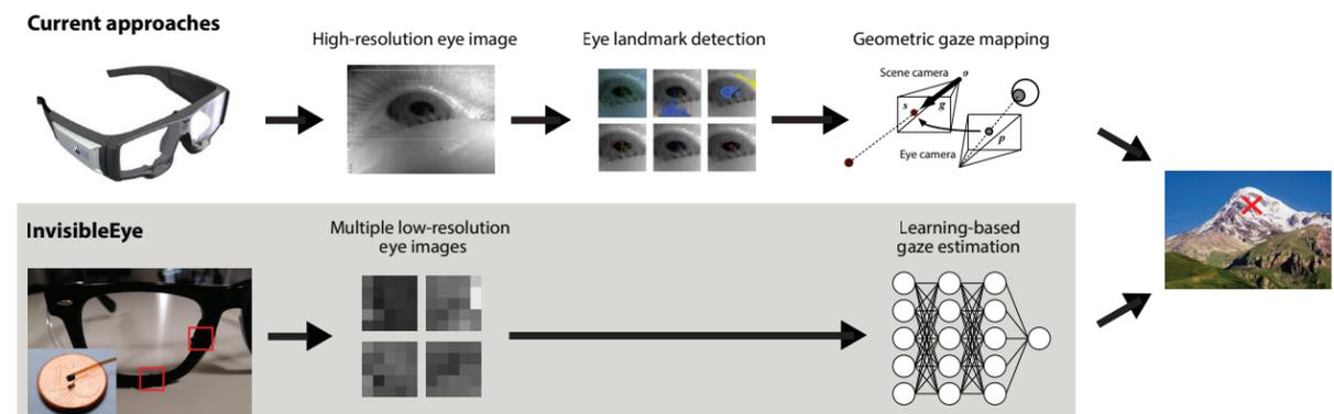
**FIGURE 1.** (Top) Classic approaches require high-resolution imaging sensors, resulting in rather bulky and obtrusive headsets, as well as hand-optimized algorithms for eye landmark
