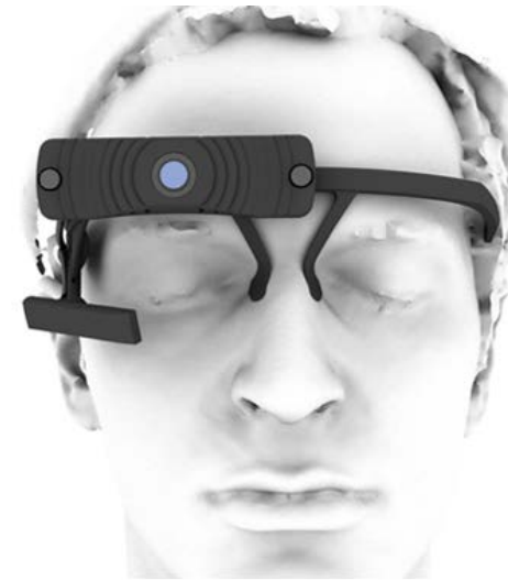
Figure 1: Front rendering of the Pupil Pro headset (rev 20) showing the frame, tiltable scene camera and adjustable eye camera.
