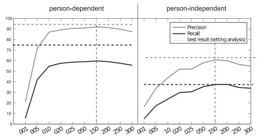
Fig. 12. Recognition performance for different subsets of the feature ranking averaged over both participants. The dashed line indicates the recognition performance only using mean and variance.
