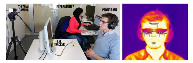
Fig. 2. Left: Experimental setup consisting of thermal camera and eye tracker facing the participant. Right: The facial features being monitored by the thermal camera (forehead, nose, left cheek, right cheek and chin).
